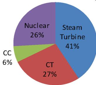
**Figure 3.** Thermal generation capacity by technology in Illinois, 2006. ST includes mainly coal-fired units, but also two residual fuel oil (no. 6) and three natural gas units. CT includes mainly natural gas-fired units, but also nine distillate fuel oil (no. 2 and jet fuel) units. CC units are natural-gas fired only.
